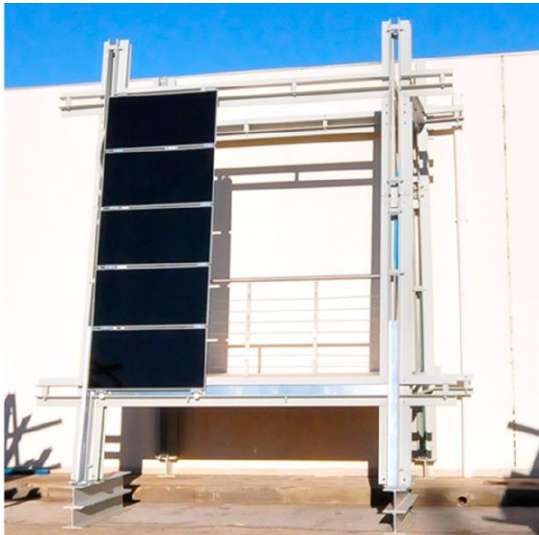
Dissipative frame exoskeleton with integrated photovoltaics Foti et al. (2020)
